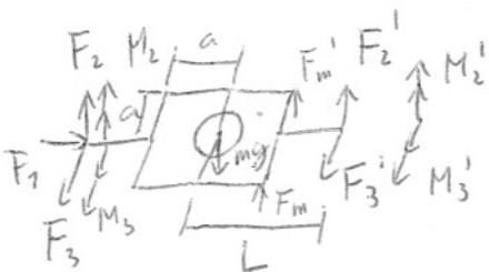
$\tilde{F} = \begin{bmatrix} F_1 \\ F_2 + F_3' + F_m + F_m' - mg \\ F_3 + F_3' \end{bmatrix} \tilde{M}^{\tilde{x}} = \begin{bmatrix} F_m' a - F_m a \\ F_3 L - F_3' L + M_2 + M_2' \\ M_3' + M_3 + F_m' a + F_m a t \\ + F_3' L - F_2 L \end{bmatrix}$
