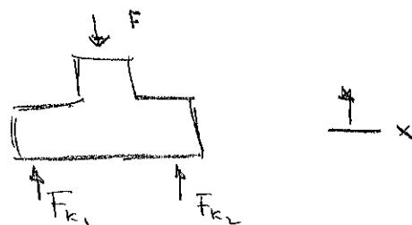
$$F_{k_1} + F_{k_2} - F = 0 \quad (\text{Como } F_{k_1} \neq F_{k_2} \rightarrow \text{P.B. EST. INDETERMINADO})$$
